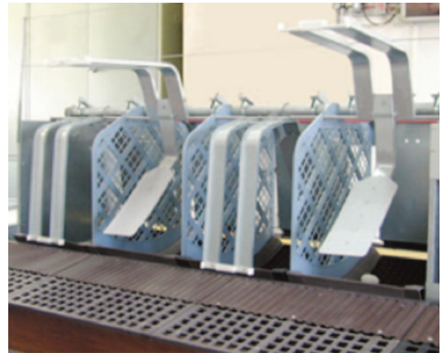
Figure 21. Example of an automatic nest box system showing ramps and "push-off" mechanisms (Courtesy of MGH)
